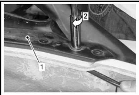
1. Grab handle 2. Handle bolt installation
