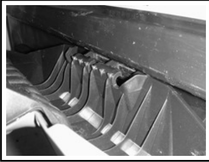
WAKE SUPPORT AFFIXED TO LOWER ANCHOR
