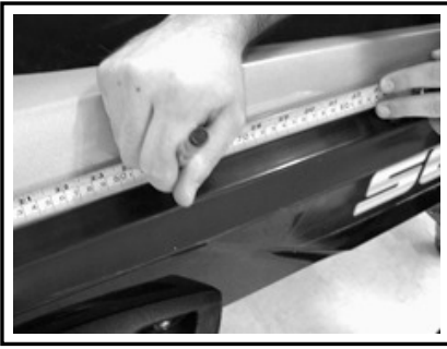
MEASURE AND MARK DISTANCE FROM REAR BUMPER
