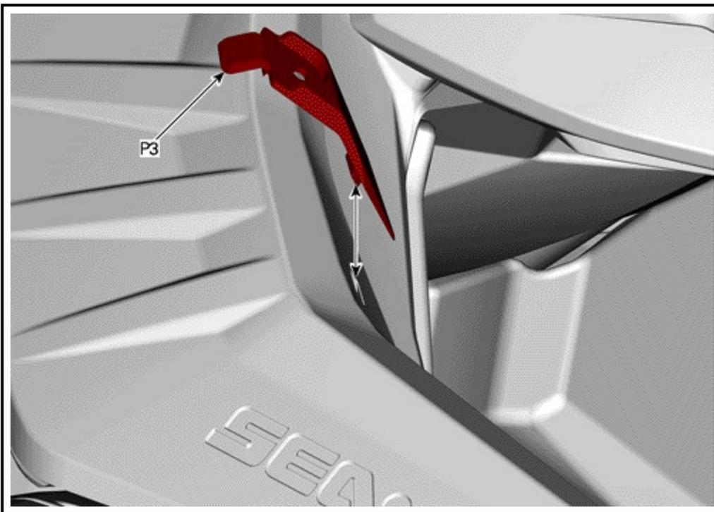
5. Drill a 5.5 mm (7/32 in) hole into body using [T1]. Use RH hook [P3] as template and secure it with a M6 x 30 Plastite screw [P5].
